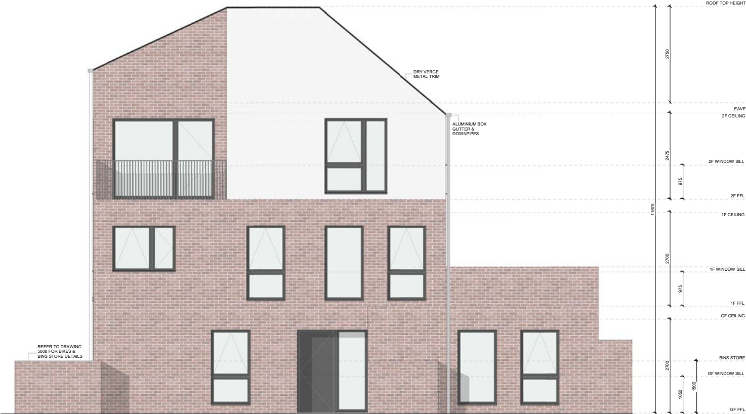
TRIPLEX T1 - MATERIALITY - FRONT ELEVATION 01 1 : 50
