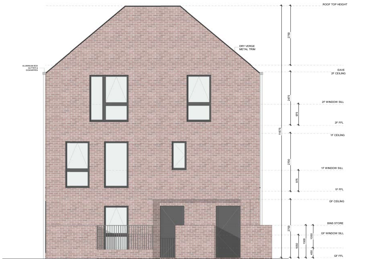
DUPLEX D1 - MATERIALITY - FRONT ELEVATION 1:50
